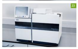
Preparative **chromatograph BUCHI Labotechnik AG SEPACORE X10** [25] with a UV detector and fraction collector. Sepacore flash chromatography system X10 addresses most requirements for purification of organic compounds. The system offers optimal performance and scale-up capability of purification of crude synthesis mixtures and plant extracts.
