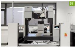
**Drop Shape Analyzer** — **DSA100E** [51] enables measurements of the surface tension of a liquid without changing **over** the instrument. This can be carried out manually or even incorporated into an automatic measuring sequence. Joint interpretation of data for liquid and solid state enables a comprehensive characterization of the component compatibility. For example, it is possible to determine the intensity of adhesion and long-term stability of a coating.
