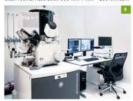
ple size. Up to 180 mm/minute writing speed. 405 nm exposure wavelength.
