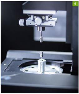
Scanning electron microscope with analytic FEI Quanta 250 FEG [5]. High resolution FEG-SEM with ESEM end STEM technology. Characterisation of conductive and non-conductive samples with SE and BSE imaging possible in every mode of operation. Resolution in high vacuum 0.8 nm at 30 kV (STEM), 1.0 nm at 30 kV (SE), 3.0 nm at 1 kV (SE); low vacuum 1.4 nm at 30 kV (SE), 3.0 nm at 3 kV (SE); extended vacuum mode (ESEM) 1.4 nm at 30 kV (SE).
