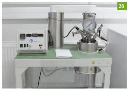
Reaction setup for processes in supercritical CO<sub>2</sub> [29]. It can work with pressures up to 350 bar and temperatures up to 350°C, its capacity is 100 mL and it is fully automated. The setup permits running of flow-through and cyclic processes. Thanks to the use of sapphire windows the processes can be controlled by spectroscopic methods. The setup includes a pump for carbon dioxide and a pump for dosing reagents under high pressure.
